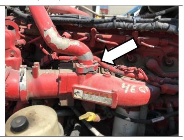
1900098 exhaust pipe and 99502-0588 clamp can used to fabricate a downpipe.
