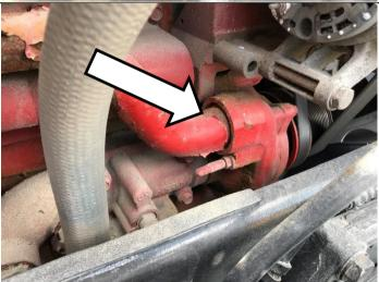
Press fit the 1900089 oil drain adapter into the engine and install the 1453106 oil drain from the turbo into the adapter. Besure to use O-ring grease on the oil drain.
